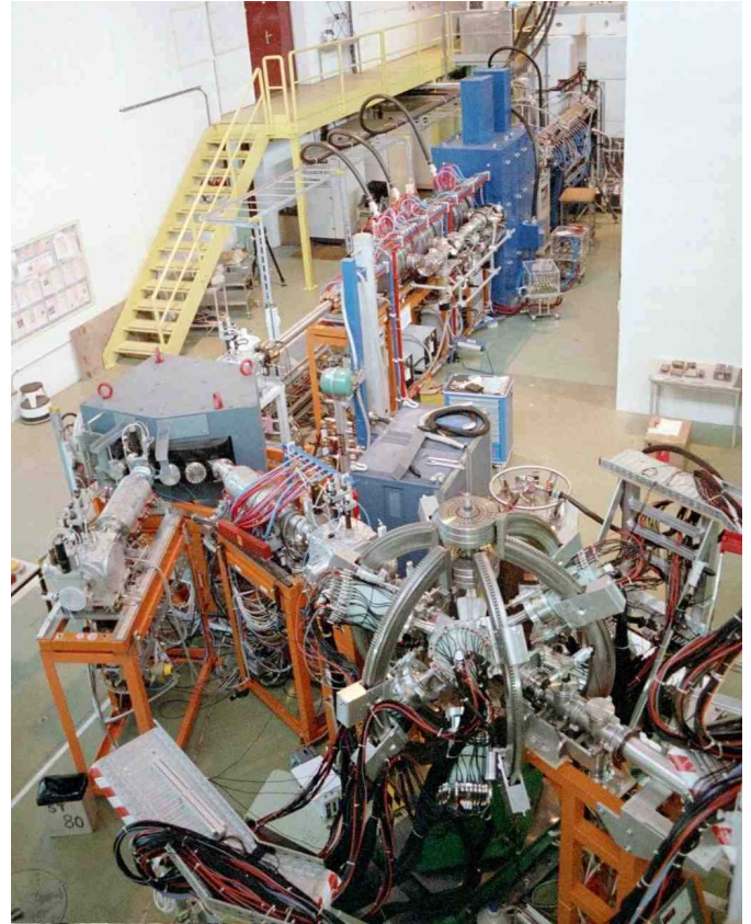
Fig. 1. The REX-ISOLDE experimental hall in 2002. In the background the REX accelerator can be seen. After the bending magnet at the 65^\circ the MINIBALL array is installed.
